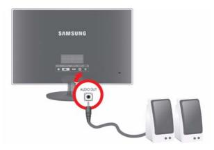
This product won't make any sound when only the HDMI cable is connected without a speaker connected.
